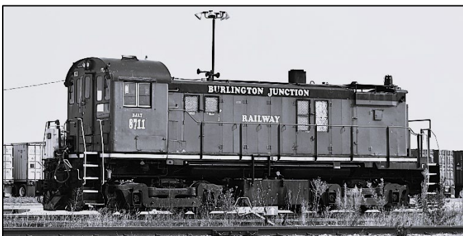
Burlington Junction’s locomotive roster has a few surprises on it, like this MLW-built former CN S13.
